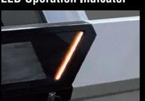
An LED operation indicator on the front of the NIRAMI allows operators to see the machine status at a glance.
