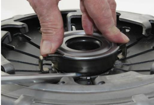
To release the bearing from the cover, apply pressure to the top of the bearing until the bearing moves very slightly downwards and insert a flat head screwdriver in between the bearing and the sprung retaining clip.
