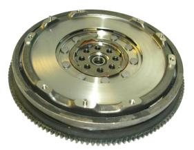
The DMF acts as a damper between the crankshaft and the input shaft on the gearbox. DMFs are made of two parts connected to a central friction ring that allows slip between them.
