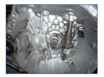
Always ensure that the bellhousing is throughly cleaned before fitting a new clutch
