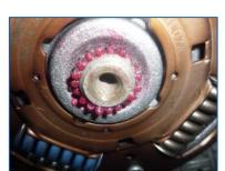
Slide the friction disc onto the input shaft
