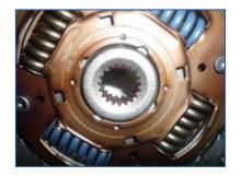
Ensure all excess grease is removed from both sides of the spline hub
