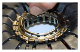
Turn the cover over and place the wire ring around the retaining clips.
