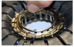
Turn the cover over and place the wire ring around the retaining clips.
