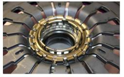
Ensure that the wire ring is seated correctly.
