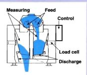
The two measuring hoppers are thus alternately filled, measured and discharged and the accumulated weight and throughput are calculated.
